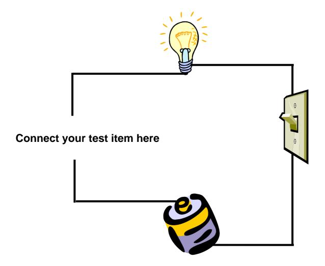
Extend the experiment by trying it out with the graphite core of an old pencil. This will show that there are some materials that are not metals and will conduct electricity.
